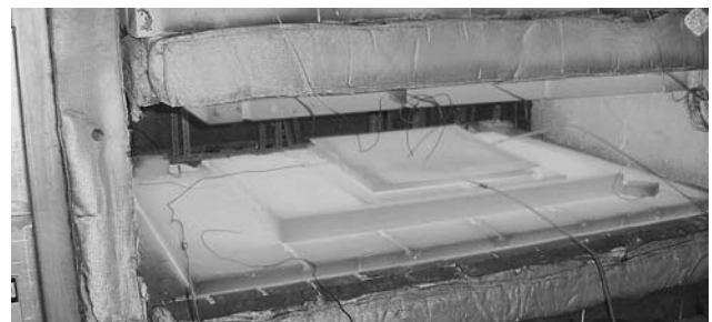
Fig. 2 Bonding of a titanium pack using a pressure bladder
