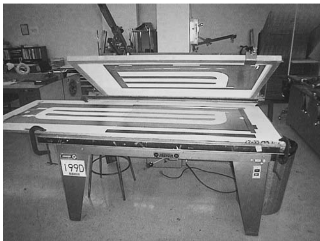
Fig. 3 Typical silk screening set-up for applying stop-off
