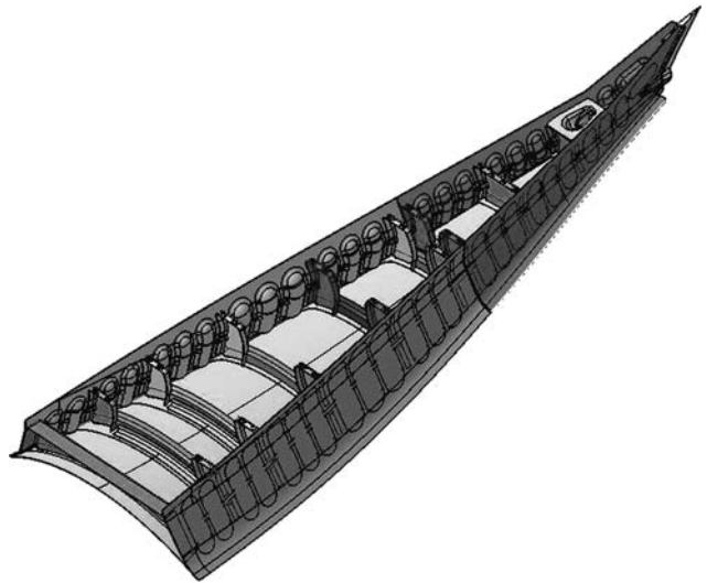
Fig. 11 Engine Aft Fairing Heat Shield Assembly using SPF/DB side panels (Ref 10)
